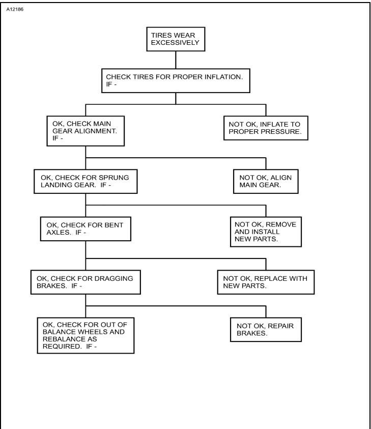
Figure 101 : Sheet 2 : Main Landing Gear Troubleshooting Chart
